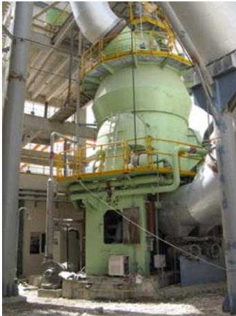
A LOESCHE mill type LM 35.3 D at Ras-el-Kaimah, U.A.E.
