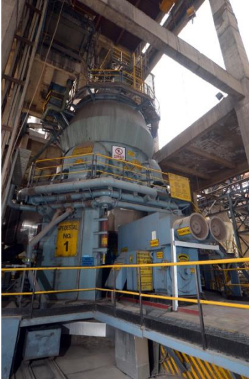
A LOESCHE mill type LM 43.4 D for grinding pet coke in Kotputli, India.
