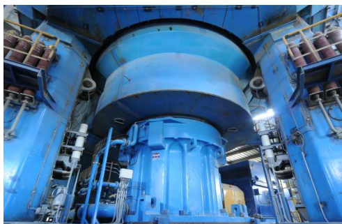
Gearbox of the LOESCHE mill in operation in the cement plant Banyuwangi, Indonesia
