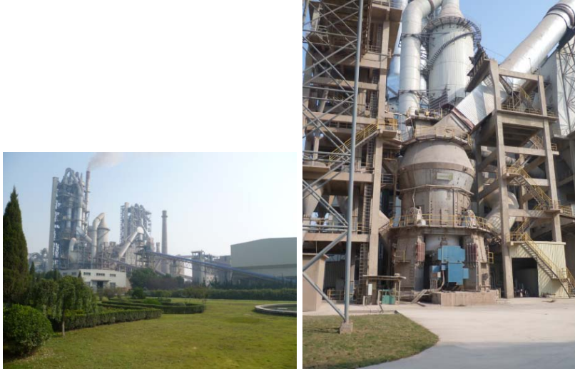
Similar LOESCHE mill of type LM 56.4 in the Jurong Cement Works, China
