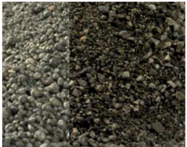
Heavy product (metal) & light product after dry density separation (-2mm)
